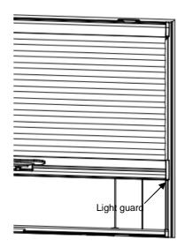
b. When light guard exceeds certain length, it will be spliced into 2 pieces. We recommend that the seam be placed as close to the fabric stack as possible, shown in below drawings.
